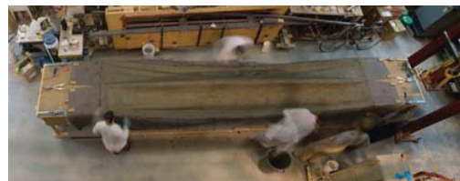
11. A flat sheet of fabric, loaded with a thin layer of concrete, self-forms itself into a funicular compression-shell mold (shown in fig. below). CAST Lab/Studio, University of Manitoba. 2009
