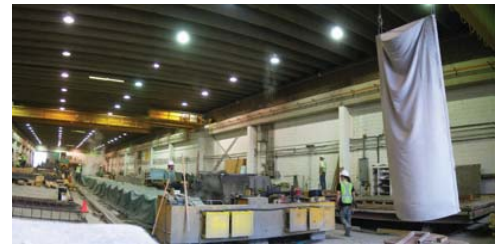
1. Fabric-formed thin-shell concrete "curtain wall" panel. Lafarge Precast Factory, Winnipeg. 2007
