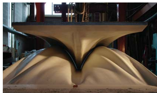
12. Fabric-formed thin-shell mold and funicular compression thin-shell cast from this mold. The deep buckling-resistant “corrugations”, that are spontaneously formed along principle lines of tension stress in the fabric mold, provide buckling-resistant “corrugations” in the compression shell cast from this mold. CAST Lab/Studio, University of Manitoba. 2009
